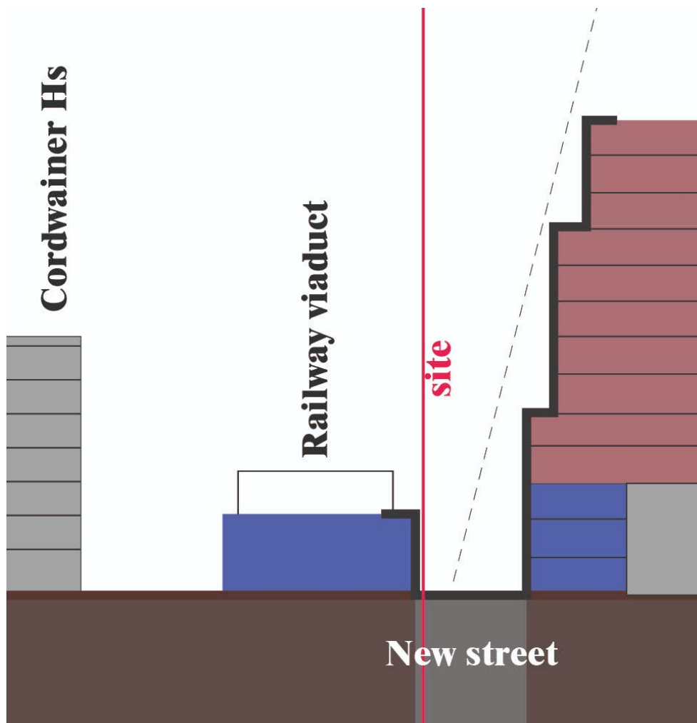
Fig X: section diagram showing an example of the railway arches a contemporary working yard and the potential relationship of street width to height of the buildings that enclose it 56
